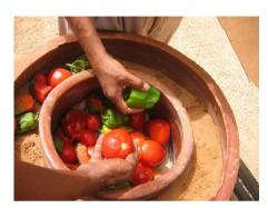
Figure 2: The Zeer pot cooling system. Photo: Practical Action Sudan.
