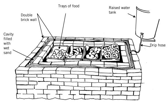
Figure 4: A static cooling system. Illustration: Practical Action / Neil Noble.
